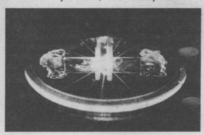
LAB ON A CHIP COMES CLOSER — A biocavity laser — a VCSEL capped by a glass plate enclosing a blood sample, all about the size of a quarter — is excited by a pump laser in Paul Gourley's lab in Bldg. 897. The VCSEL device can produce information about the state of millions of blood cells in a few minutes.
